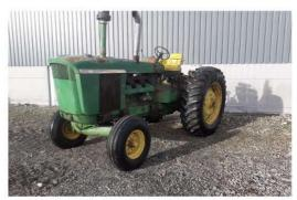
Model: 5020 Year 1967 Hours: 6057 Registration: KNT 126E Serial No: T313R 017699R IMPORTED FROM USA. TACHO WORKING. FITTED WITH 6030 ENGINE, CAB WITH DOORS & AIR CON, 2 DOUBLE ACTING SPOOLS, LINKAGE, PTO, DRAWBAR. WITH DUAL WHEELS.
